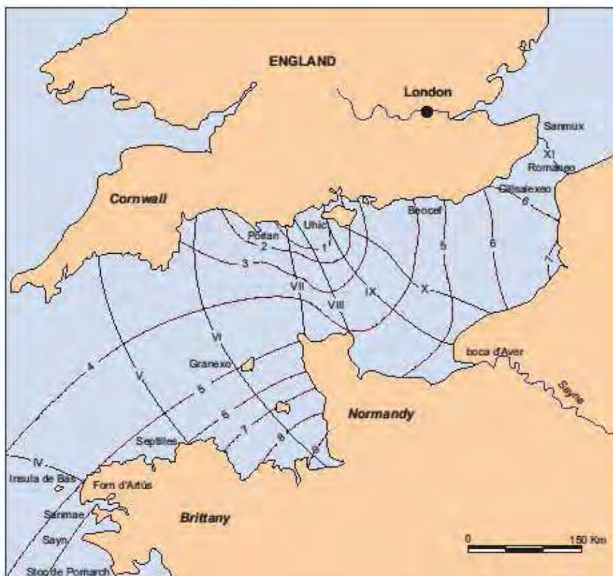
Figure 3. Map of the English Channel with the toponyms contained in the Catalan Atlas and the cotidal lines. The continuous lines represent cotidals (same tide height) in lunar time and the broken lines represent the tidal range (height difference) in metres.
